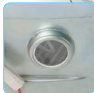
Sight Window to Combustion Chamber
